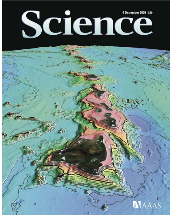
Figure 6. Seafloor depth based on ship soundings and satellite altimetry draped over matching seafloor in Google Earth (500 m contour interval) was used for the December 2009 cover of Science. The global kmz-file is available at ftp://topex.ucsd.edu/pub/global_topo_1min/global_topo_1min_V12.1.kmz .
