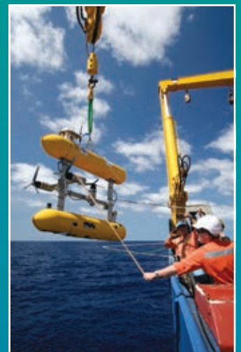
Lowering the Conductivity/Temperature/Depth profiler in the Coral Sea on the RV Southern Surveyor .
