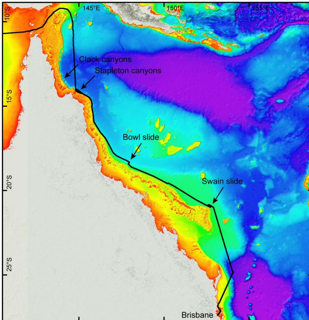
Figure 1. Plan view map of voyage IN2019\_T02 from Brisbane along the GBR slope, showing the four areas of interest: Swain slide, Bowl slide, Stapleton canyons and Clack canyons survey areas.
