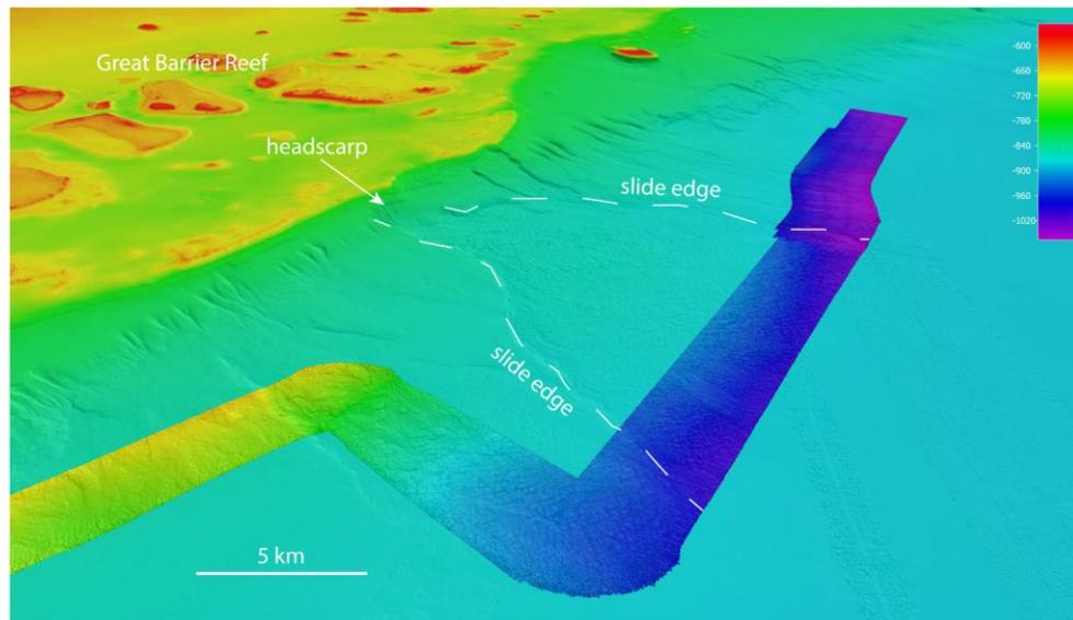
Figure 3. Westerly 3D view of the Bowl slide, showing the new multibeam data extending farther the slide debris field to ~30 km from the headscarp on the upper slope.
