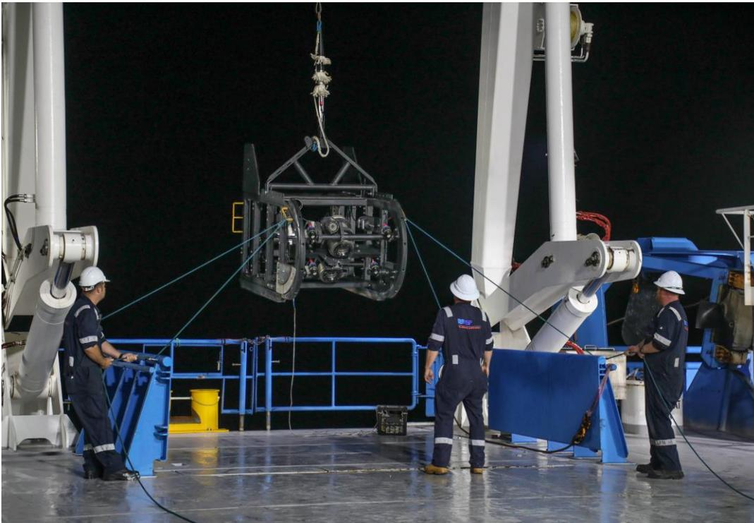
Figure 13: Deployment of the deep tow camera during the Wessel Marine Park survey (Photo: Cass Erbs/CSIRO).
